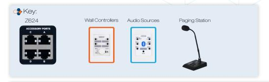
Each port supports 2 wall controllers and 2 audio sources, or 1 audio source and a paging station
